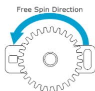
For Springs Installed at Left End of Header
