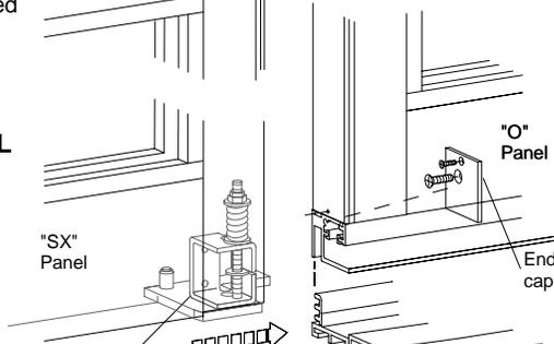
Install threshold after all panels are in place.
