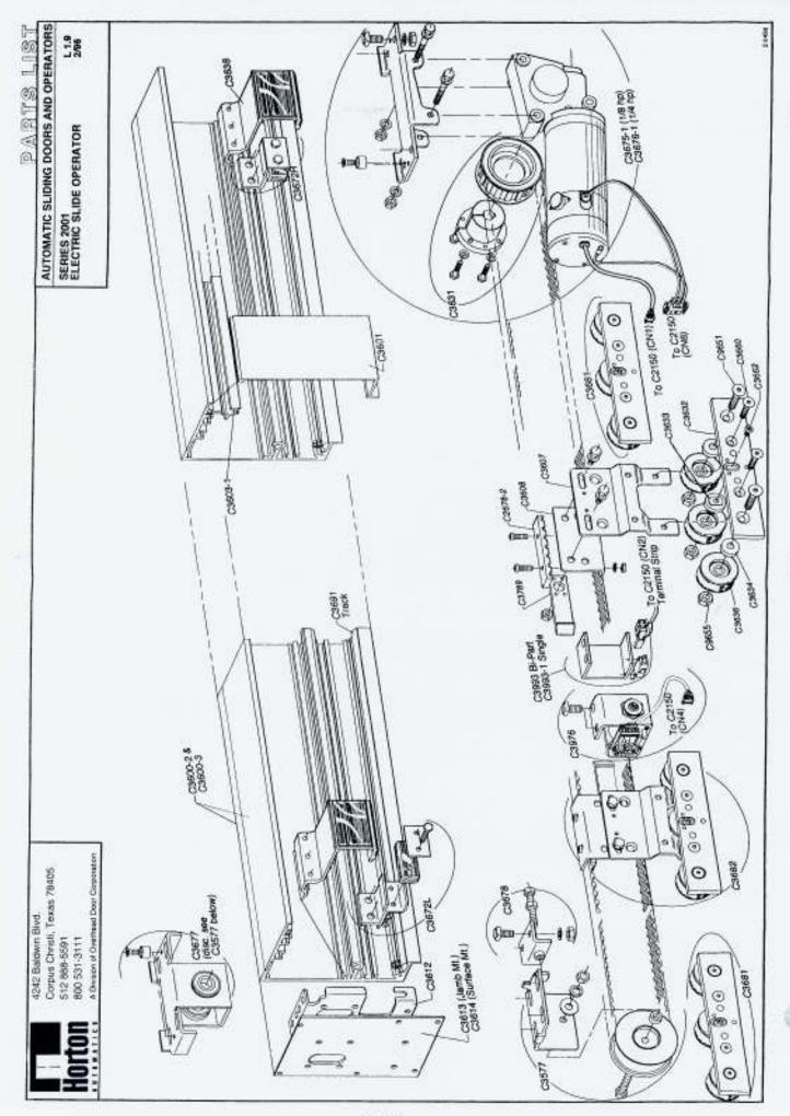
A.C. Power in All Fuses are 5x20 mm Type T 5x20 mm Type T 5x20 mm Type T C3925 Power Supply To Motor & PARTS LIST AUTOMATIC SLIDING DOORS AND OPERATORS 2796 SERIES 2001
