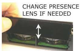
WIDE-FIELD LENS (FACTORY DEFAULT) [6'6"(W)X13.75"(D)]
