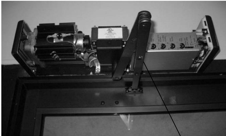
Connecting arm perpendicular to the door.
