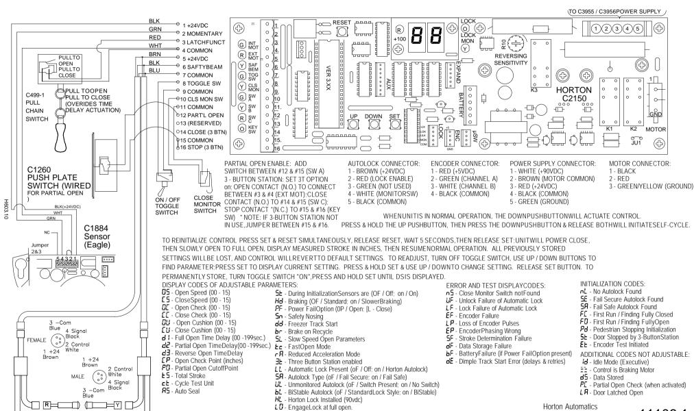
ACTUATING & CONTROL SWITCH CONNECTIONS TO C2150 INDUSTRIAL CONTROL
