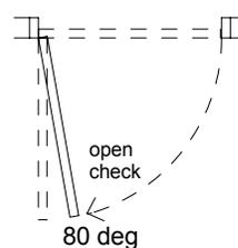
**OPENING TIME:** Doors shall be field adjusted so that opening time to open check or 80 deg shall be three sec. or more and not exceed 15 ft. lb. to prevent opening or closing.
