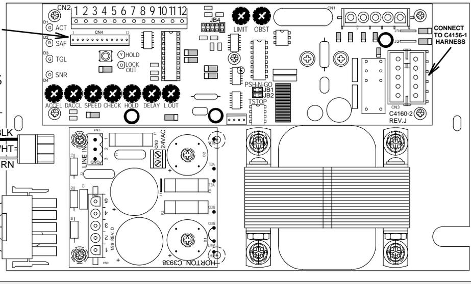
**Automatic Swing Operator Wiring with C4190 Control REV."J"11380.8**
