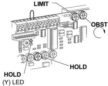
If a presence detector is installed on the swing side of the door, an obstruction response will "hang up" the presence detector and the door, until the door can get to the full open position.
