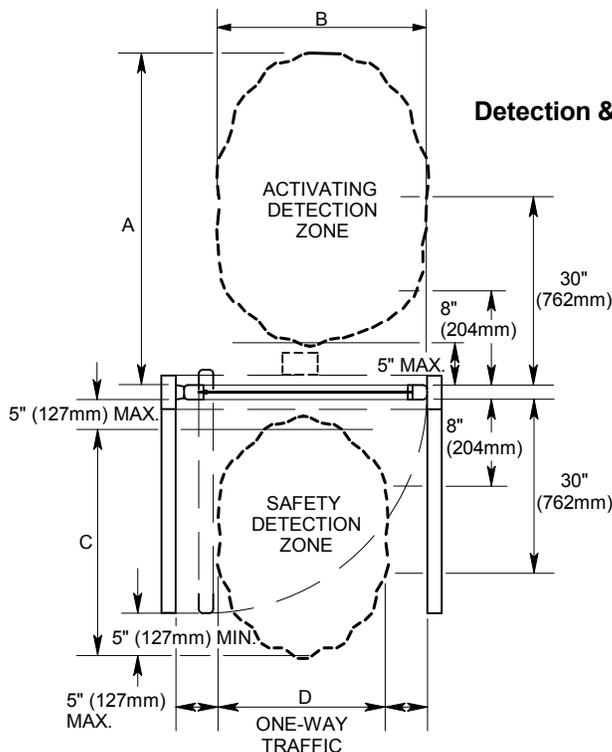
**Detection & Safety Zones - Header Mounted Safety Sensors**
