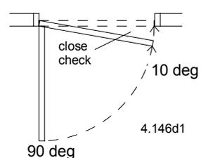
**CLOSING TIME:** Doors shall be field adjusted to close from 90 to 10 deg in three sec. or longer. Doors shall close from 10 deg to fully closed in 1.5 sec. or more.
