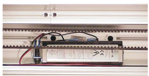
Plug the cable into the mating 3-conductor connector located on the lower right of the operator control.
