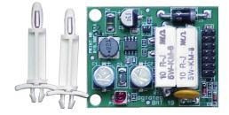
9-51-0016 Charger/Monitor Circuit Board for 9-51-0017 Lead Acid Battery Assembly
