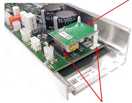
LOCATE CONNECTOR AND SPACER HOLES FOR THE LEAD ACID CHARGER/MONITOR CIRCUIT BOARD
