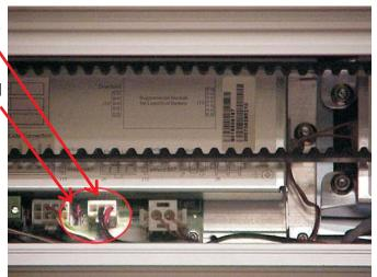
This will reset the control and it will reconfigure properly for the battery module.
