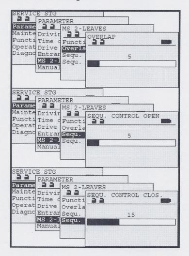
7 – REMOVE PROGRAMMER, PUT SWITCH TO "AUTO" AND ACTIVATE DOOR. TEST FUNCTION OF DOOR. ADJUST SETTINGS AS NEEDED.
