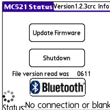
**Step 3:** Turn on power to the Bluetooth Programming Adapter. Run the MC521 Toolbox application. Select the **Bluetooth** button. The **Bluetooth Discovery Results** screen shall be displayed.
