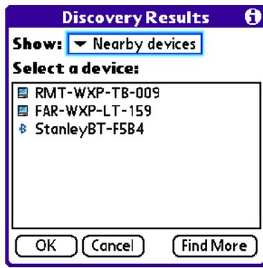
**Step 5:** On the Bluetooth **Discovery Results** screen, select **Nearby Devices** from the **Show** dropdown list. The Bluetooth Programming Adapter shall be listed as StanleyBT-XXXX, where XXXX are the last four digits of the serial number on the unit label. Select the Bluetooth option and click **OK**.
