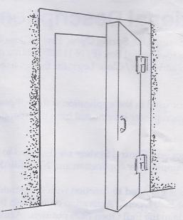
Doors must swing freely on hinges or pivots of adequate size for good automatic door operation. The doors, even though not supplied by Stanley, must be checked for the following items as they influence the operation of the automatic door equipment:
