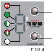
Browse through the fault display using selector key 1 upwards (to display several faults).
